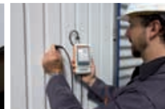
Measurement of a paint coating on steel
