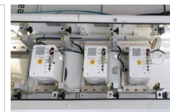
Simultaneous measurement by several FISCHERSCOPE® X-RAY 5100
