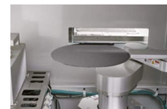
Handling robot loads measuring device with wafers
