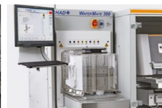
Automatic docking and loading of wafers in standardized FOUPs and cassettes
