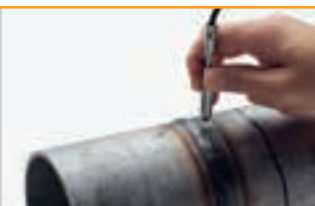
FERITSCOPE® FMP30: Ferrite content measurement on weld seams
