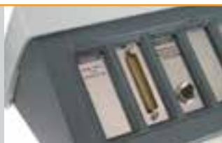
Back of the MMS PC2. Eight module slots are available.
