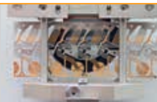
Sensor contacts: Au/Ni/CuFe
