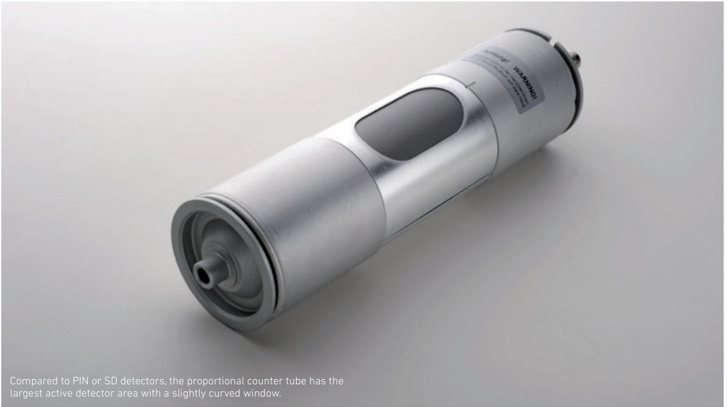
Compared to PIN or SD detectors, the proportional counter tube has the largest active detector area with a slightly curved window.
