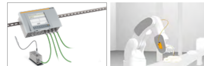
Measuring module and probe are mounted directly on an inline measuring station (left illustration) or a robot (right illustration)
