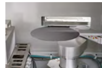
Handling robot loads measuring device with wafers
