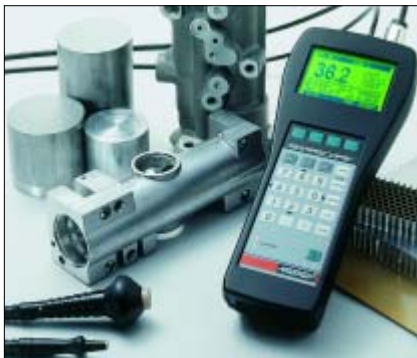
SIGMASCOPE® SMP10 for the measurement of the electrical conductivity of metals. The measurement results permit statements about the composition, microstructure and mechanical properties of the specimen.
