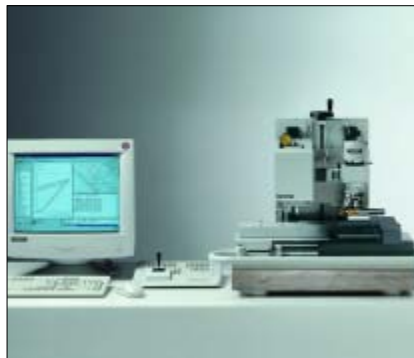
Micro hardness measurement unit FISCHERSCOPE® HIM2000 to determine the Martens hardness of thin coatings and foils.
