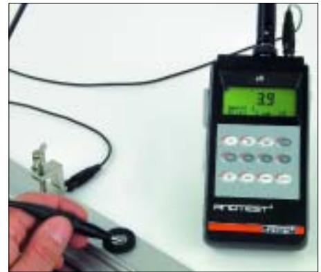
ANOTEST® YMP30-S with grounding cable and grounding clamp, meas. electrode and meas. cell.
