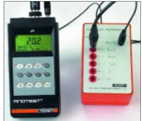
Accurate electr. reference for the calibration of the ANOTEST® YMP30-S.
